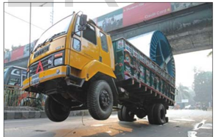
Fig 4: Over height Truck stuck with Ramna footbridge
